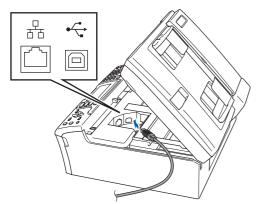
Carefully route the USB cable through the trench and out the back of the machine as shown below and connect the cable to your Macintosh<sup>®</sup>.
